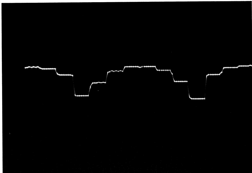
Fig. 2. a) Output of the logarithmic full-wave rectifier with a sine wave at the input b) The same signal after sampling
